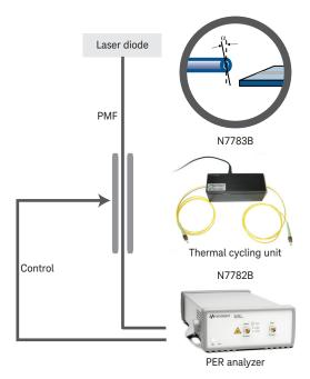
Figure 1. Laser diode pigtailing using the combination of N7782B and N7783B.
